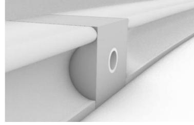
Figure 1.15 Indicative stormwater outfall penetration through seawall.
