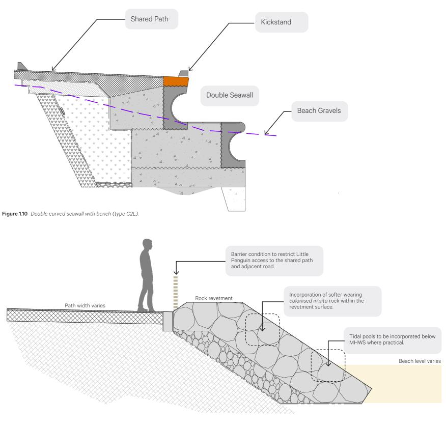
Figure 1.11 Typical rock revetment section.
