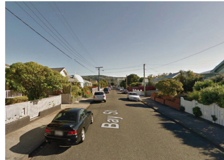
Bay Street: Typical 3a street pattern, narrower street width (7.5m) than 3b (14m). Plot-to-plot widths 12m (3a), 20m (3b). No street trees, planting on plots.
